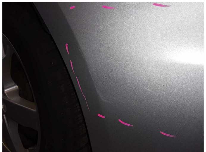
Damage 5: Rear bumper: Rear bumper - Scratch(es) - Paint
