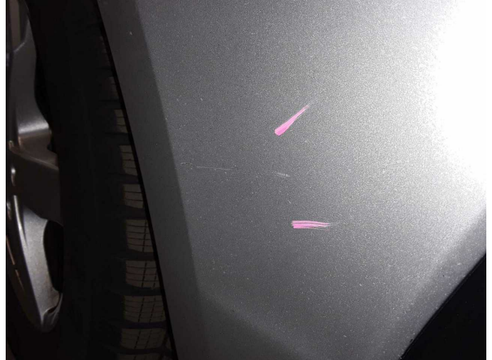
Damage 4: Front bumper: Front bumper - Scratch(es) - Paint
