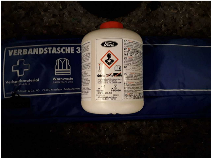
Damage 1: Equipment: Tirefit filler - Expired - Replace
