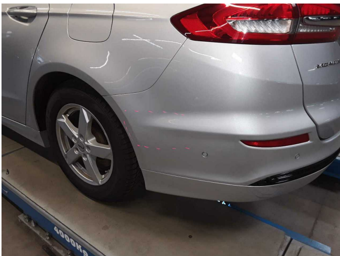
Damage 5: Rear bumper: Rear bumper - Scratch(es) - Paint
