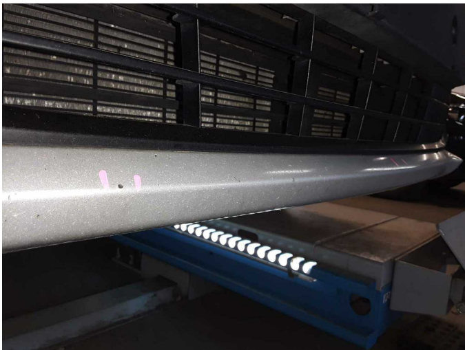
Damage 4: Front bumper: Front bumper - Scratch(es) - Paint
