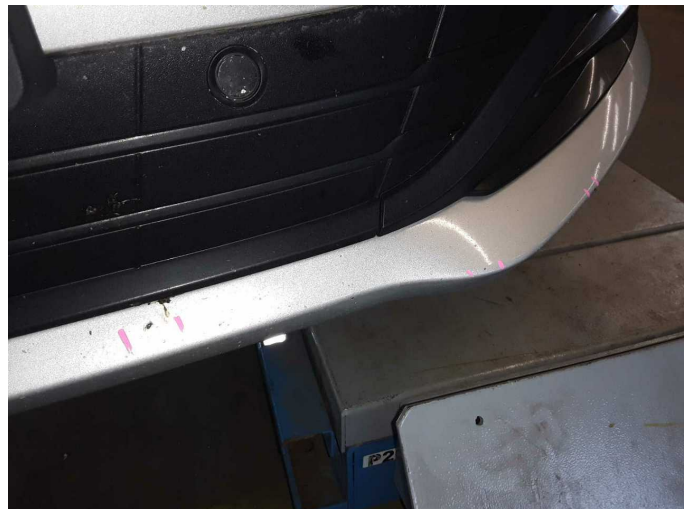
Damage 4: Front bumper: Front bumper - Scratch(es) - Paint
