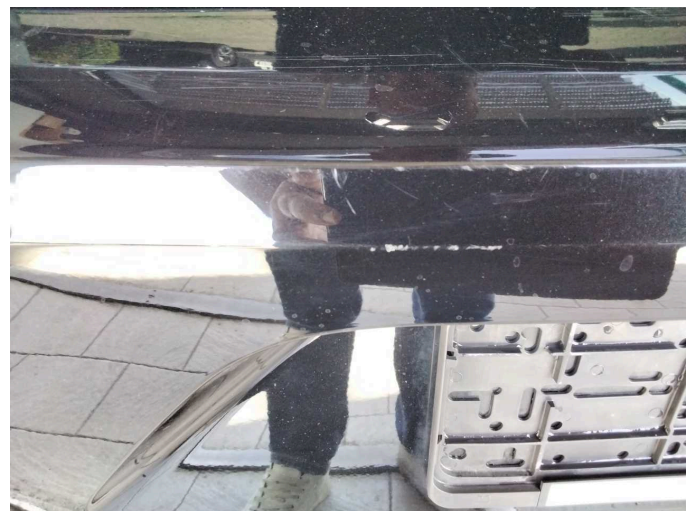
Damage 11: Rear bumper: Rear bumper - Scratch(es) - Paint
