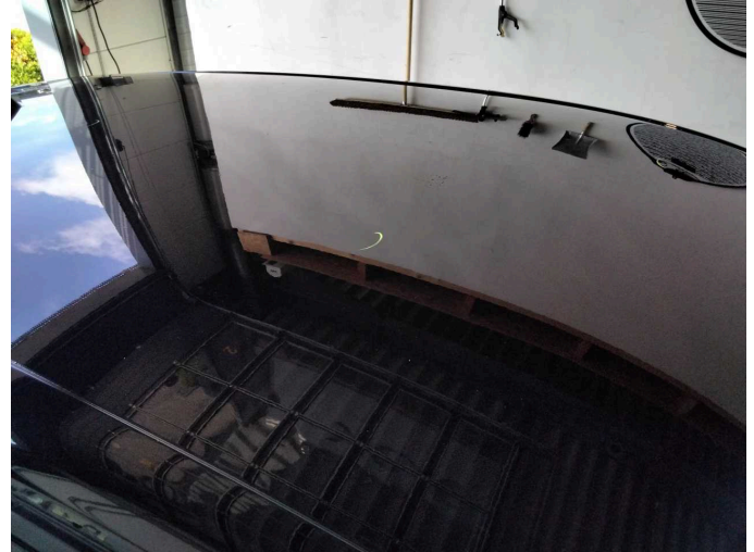
Damage 7: Roof: Roof - dent(s) - Smooth repair work
