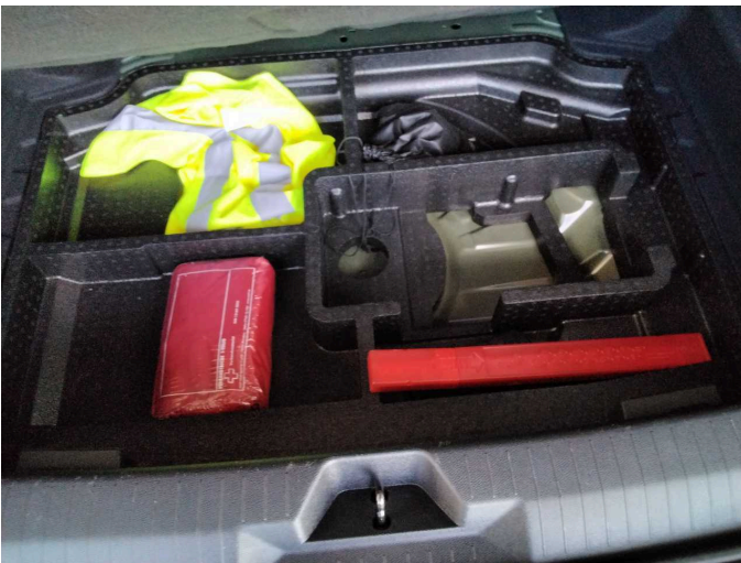
Missing part 2: Equipment: Tirefit complete - Missing - Replace
