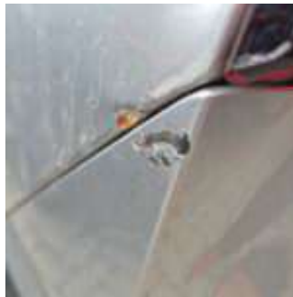
Damage Type small dents / small scratches
