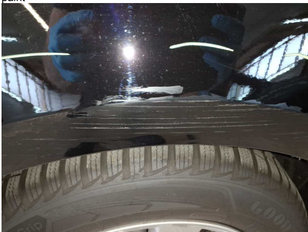
Damage #7: Side panel - rear right side: Side panel - Scratched - Repair and paint
