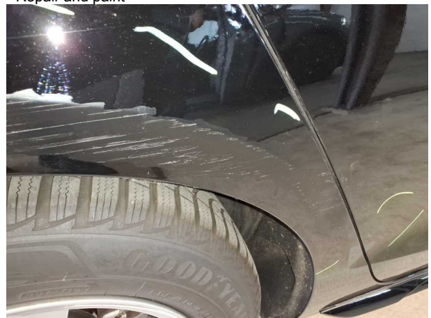
Damage #7: Side panel - rear right side: Side panel - Scratch... - Repair and paint
