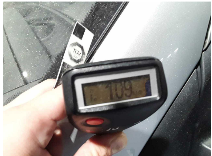
Dachholm links: 109 µm
