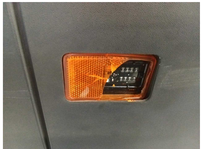
Damage 1: Indicator - front: Indicator lamp - rear right side - Broken / torn - Replace
