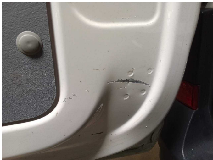
Damage 3: Boot lid / rear door: Boot lid (innen) - Dent / paintcoat damage - Loss in value
