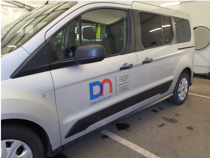
Damage 6: Body: Body - Glued / labelled - De-glue / neutralise
