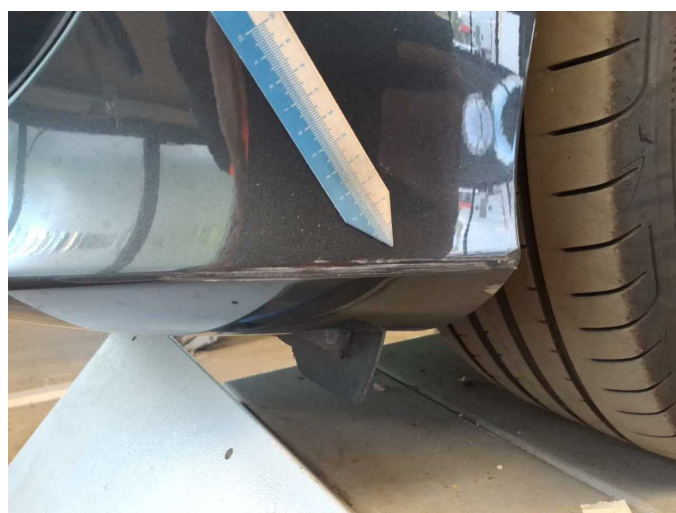
Damage 8: Front bumper: Front bumper - Scratch(es) - Paint
