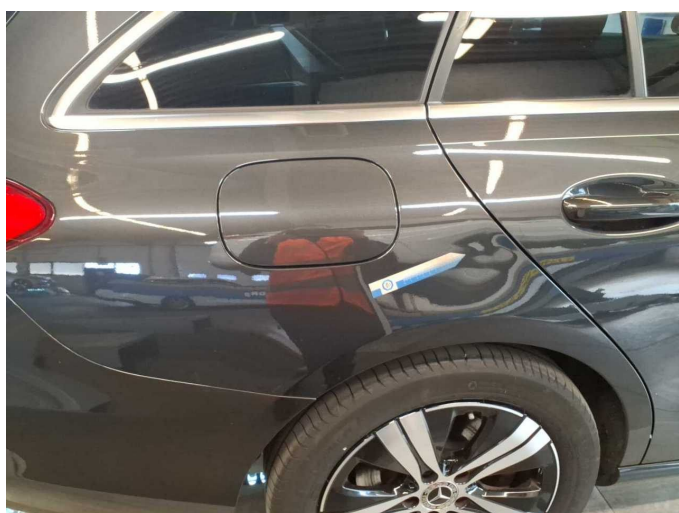
Damage 11: Side panel - rear right side: Side panel - Deformed - Repair and paint
