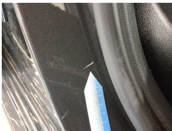
Damage 3: Sill - right side: Sill - Scratch(es) - Smart repair
