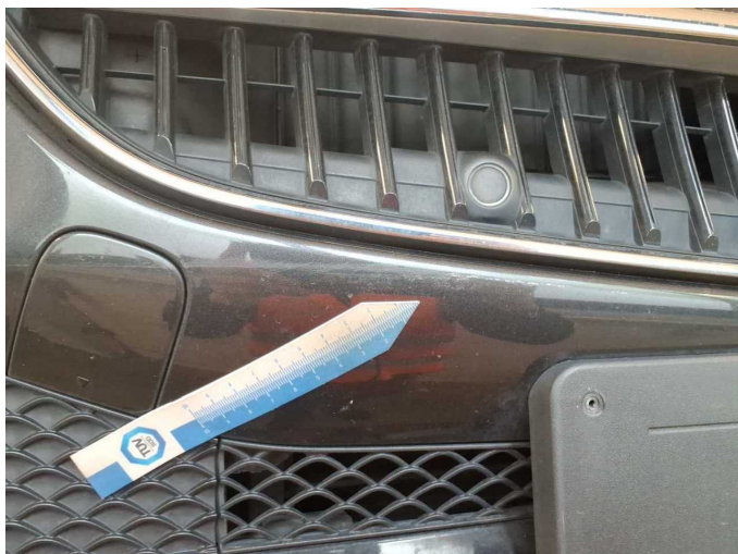
Damage 8: Front bumper: Front bumper - Scratch(es) - Paint
