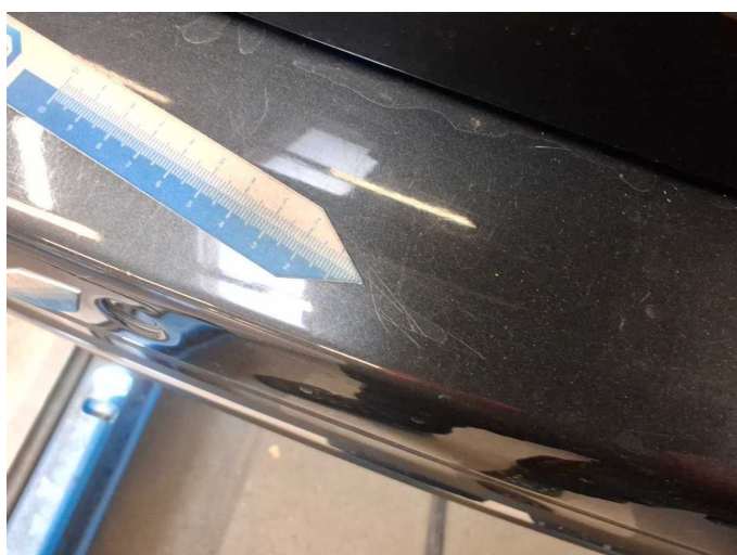
Damage 7: Rear bumper: Rear bumper - Scratch(es) - Paint
