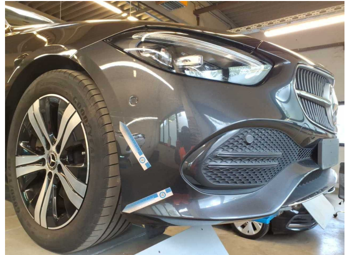
Damage 8: Front bumper: Front bumper - Scratch(es) - Paint
