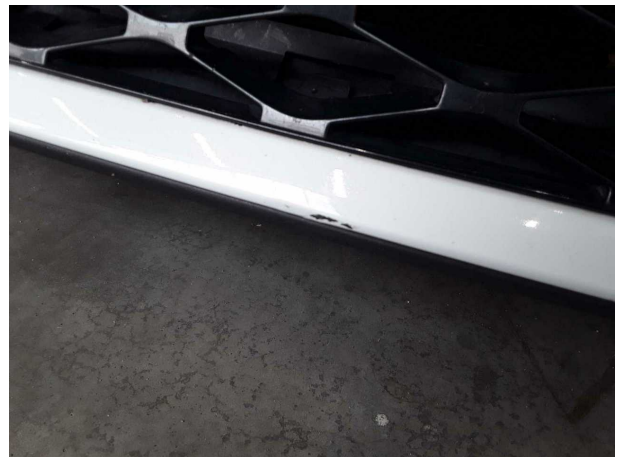
Damage #2: Front bumper: Spoiler - Scratch(es) - Paint
