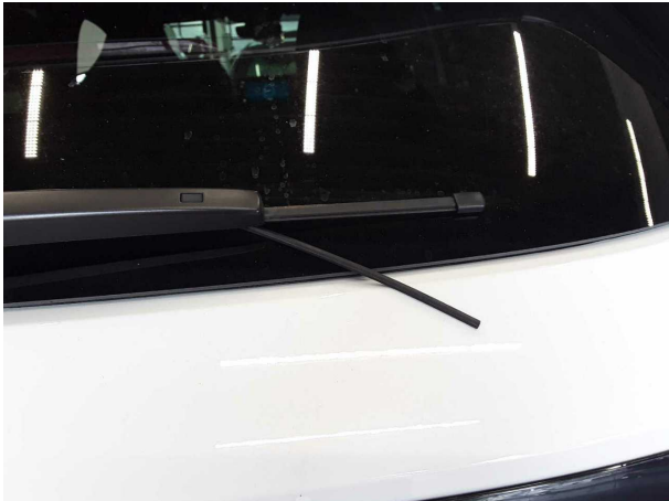
Damage #1: Screen cleaning: Wiper blades - rear - Broken / torn - Replace
