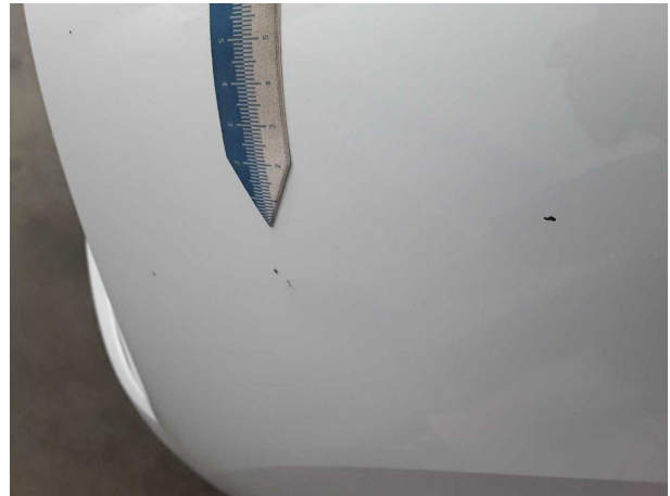
Damage #5: Front bumper: Front bumper - Scratch(es) - Paint
