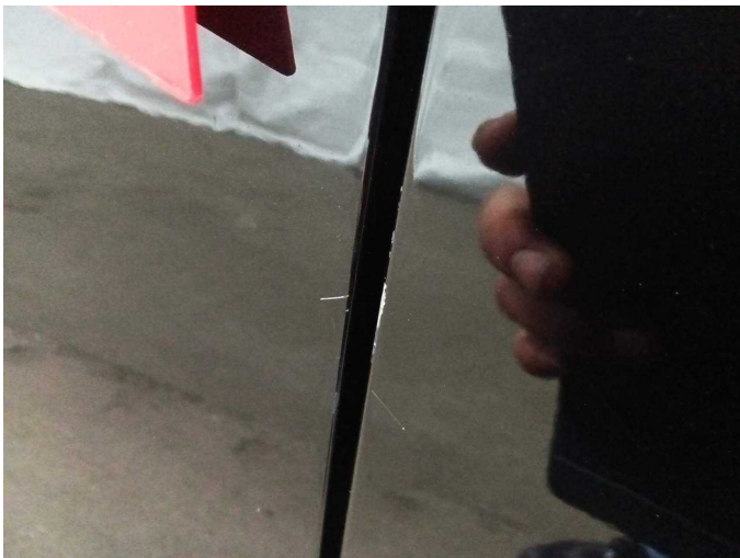
Damage 5: Sliding door, right: Sliding door - Scratch(es) - Smart repair
