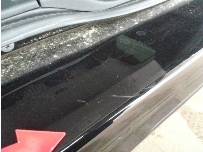
Damage 6: Rear bumper: Rear bumper - Scratched - Paint
