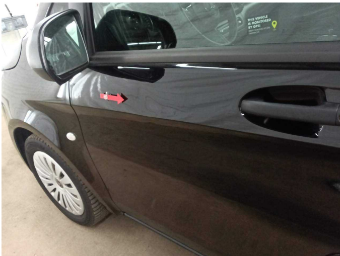
Damage 7: Door - front left side: Door - dent(s) - Repair and paint
