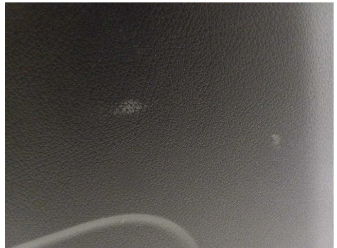
Damage 4: Trim / covers: Boot lid - interior trim - Scratched - Loss in value
