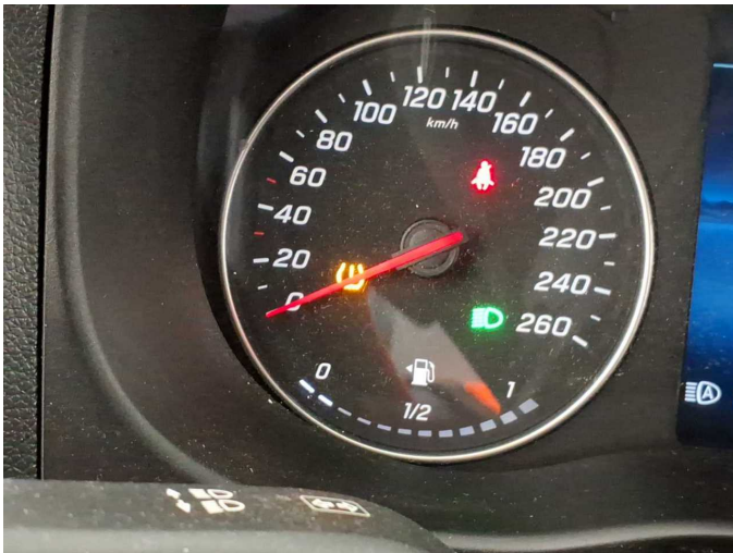
Damage 3: Instrument panel: Indicator light (Reifendruck Kontrollleuchte) - on - Perform diagnosis
