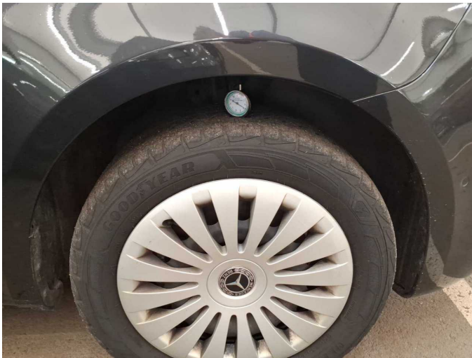
Damage 4: Wheel / tyres: Tyre - front right side - Does not meet the leasing specifications - Replace
