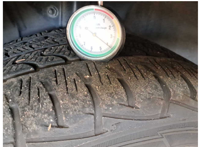
Damage 5: Wheel / tyres: Tyre - front left side - Does not meet the leasing specifications - Replace
