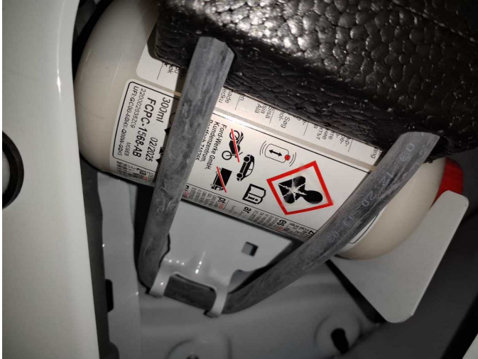
Damage 1: Equipment: Tirefit filler - Expired - Replace
