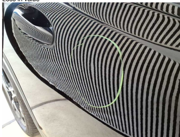
Damage #4: Door - rear right side: Door - dent(s) - Smooth repair work
