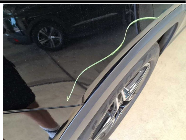
Damage #5: Side panel - rear right side: Wheel well extension - Malposition - Un- / install
