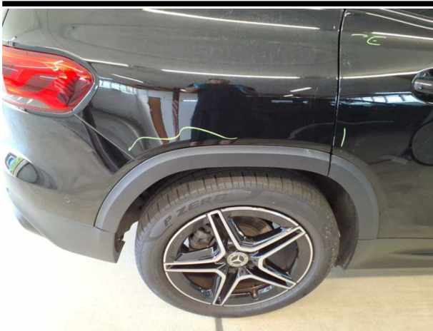
Damage #5: Side panel - rear right side: Wheel well extension - Malposition - Un- / install
