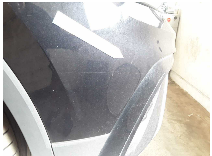
Damage 6: Front bumper: Front bumper - Scratch(es) - Paint
