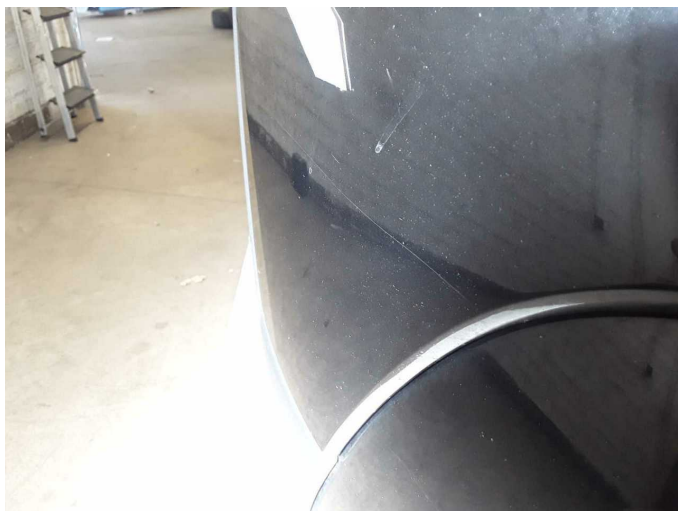
Damage 6: Front bumper: Front bumper - Scratch(es) - Paint
