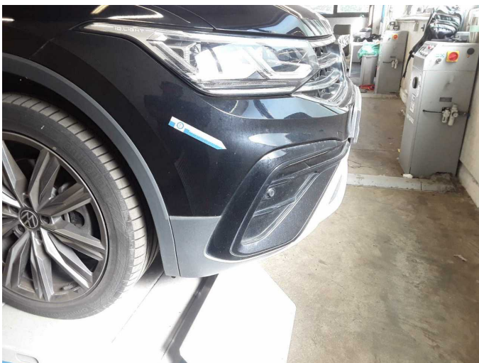
Damage 6: Front bumper: Front bumper - Scratch(es) - Paint
