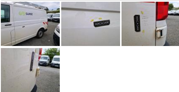
Brand badge F, Missing, Replace
