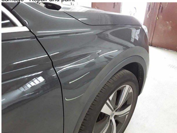
Damage #7: Mudguard - right side: Mudguard - right side - Scratched - Repair and paint
