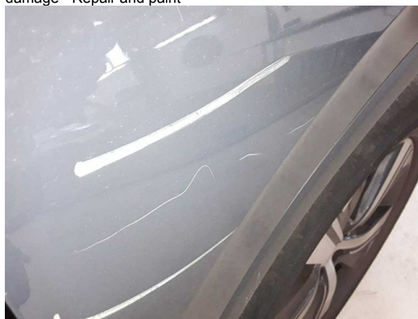
Damage #7: Mudguard - right side: Mudguard - right side - Scratched - Repair and paint
