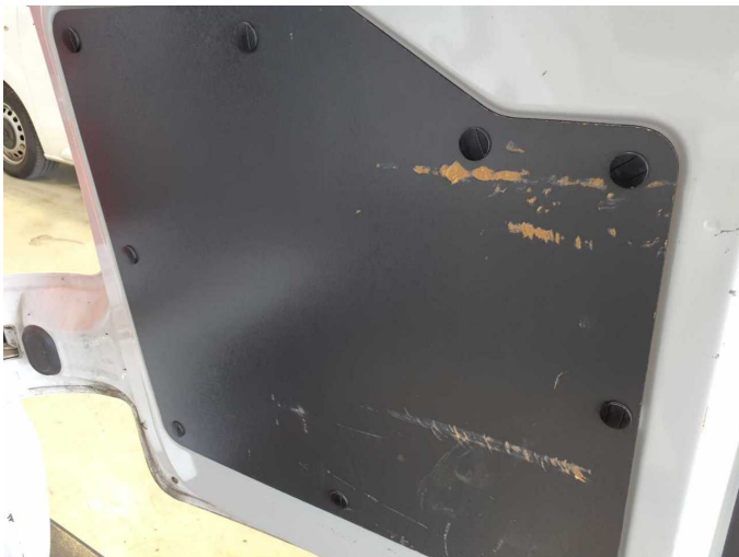
Damage 4: Trim / covers: Door trim - rear right side - Scratch(es) - Loss in value
