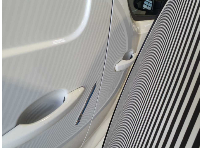
Damage 12: Sliding door, right: Sliding door - Dent / paintcoat damage - Smart repair
