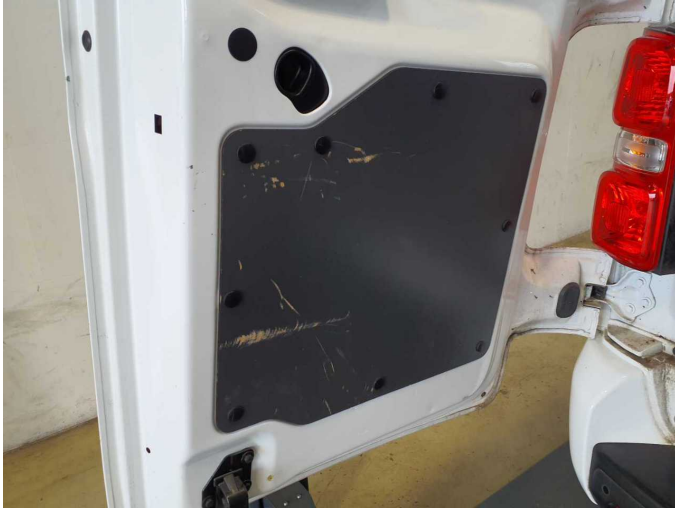
Damage 3: Trim / covers: Door trim - rear left side - Scratch(es) - Loss in value
