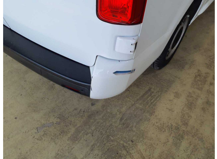
Damage 16: Rear bumper: Bumper - rear right side (Eckteil) - Broken / torn - Replace
