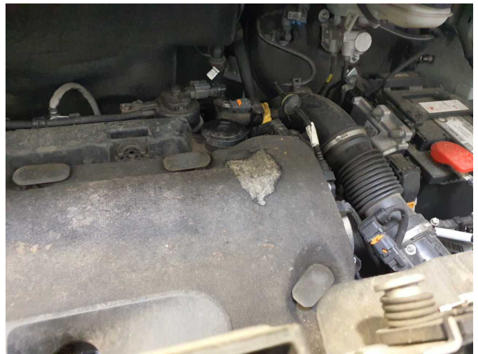
Damage 14: Engine: Engine cover - Broken / torn - Replace
