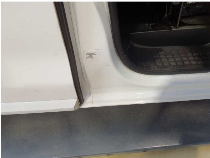
Damage 7: Sill - right side: Sill - Dent / paintcoat damage - Smart repair
