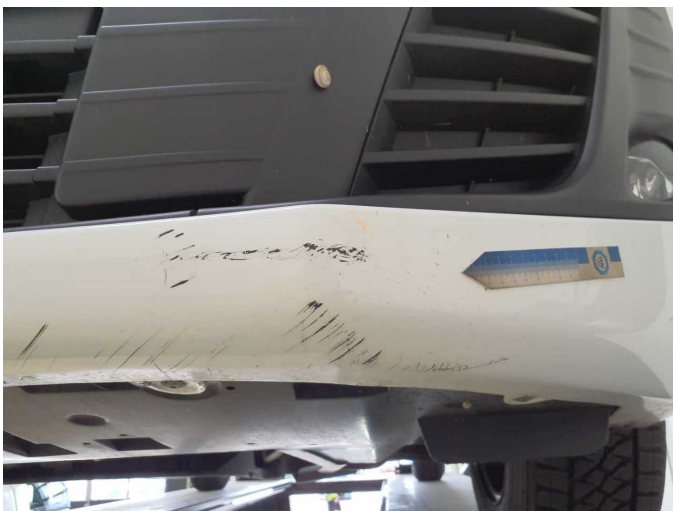
Damage 17: Front bumper: Front bumper - Dent / paintcoat damage - Repair and paint
