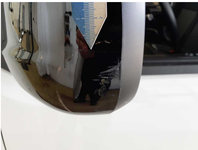
Damage 5: Wing mirror - left side: Cap - Scratch(es) - Repaired
