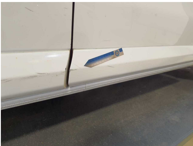
Damage 8: Door - front right side: Brightware - lower - Scratch(es) - Smart repair
