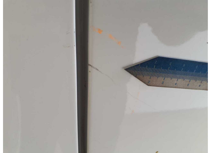
Damage 9: Side panel - rear left side: Side panel - Scratch(es) - Smart repair
