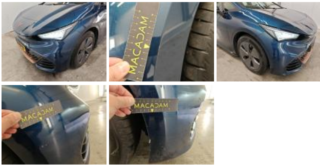
Sill trim R, Scratch(es), Repair and paint (complete)
