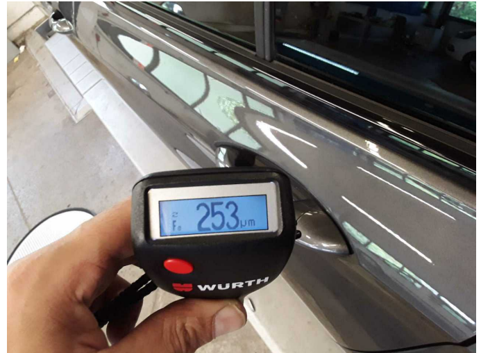
Repainting 1: Roof, Side panel - rear right side, Door - rear left side, Door - rear right side, Door - front left side, Door - front right side
