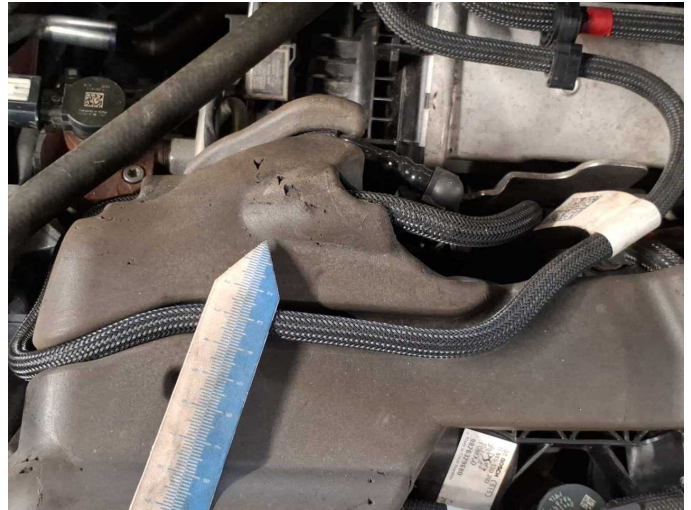
Damage 6: Engine: Hose turbocharger (+ Isolierung Motor & Dämmmatte Motorhaube) - Damage caused by marten / rodent - Replace
