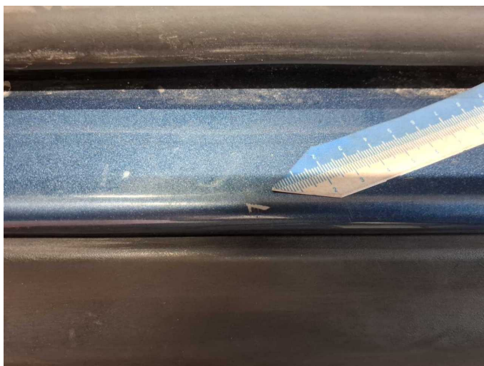
Damage 2: Sill - left side: Sill (Vorne) - Scratch(es) - Smart repair
