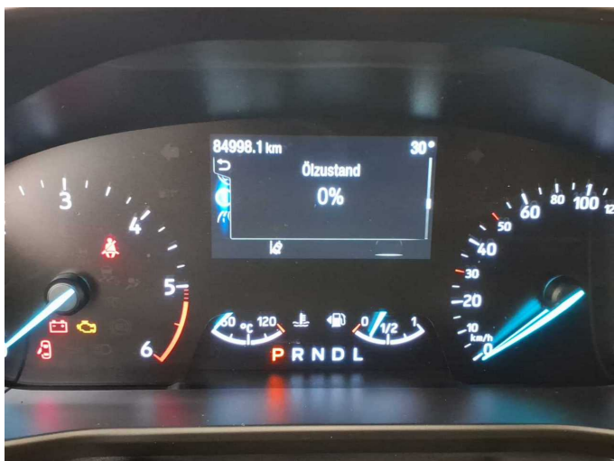
Damage 7: Misc.: Inspection / maintenance - Due - Perform
