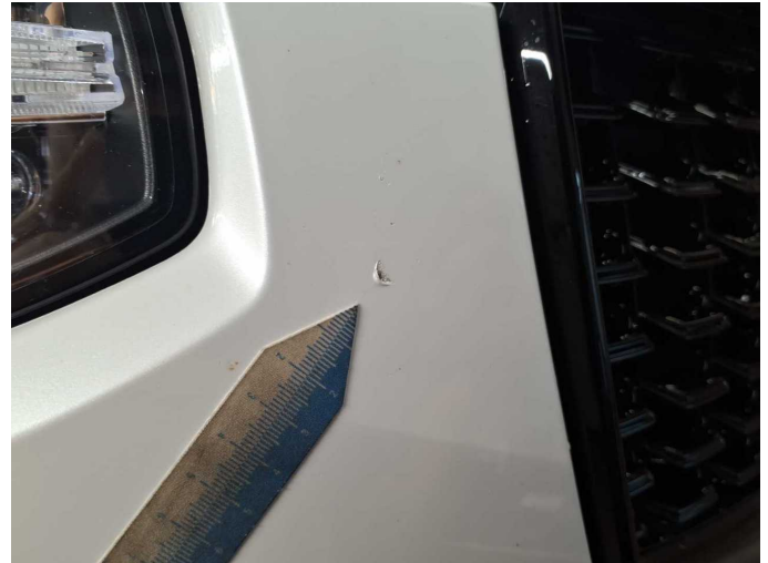
Damage 5: Front bumper: Front bumper - Scratch(es) - Paint
