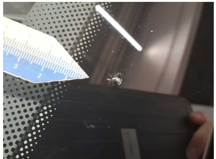
Damage 6: Vehicle glazing: Windscreen (Rand-Bereich) - Stone chips - Replace
