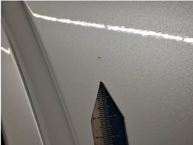
Damage 5: Front bumper: Front bumper - Scratch(es) - Paint
