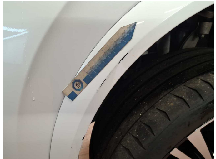
Damage 4: Mudguard - left side: Wheel well extension - Scratch(es) - Paint
