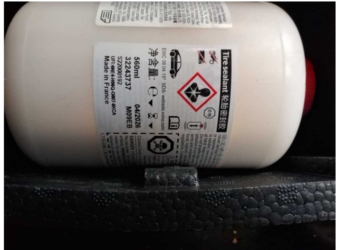
Damage 1: Equipment: Tirefit filler - Due - Replace
