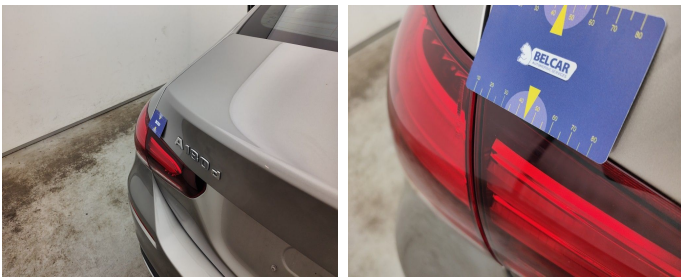
Light / Rear Left On Rear Bonnet / Replace-scratch
