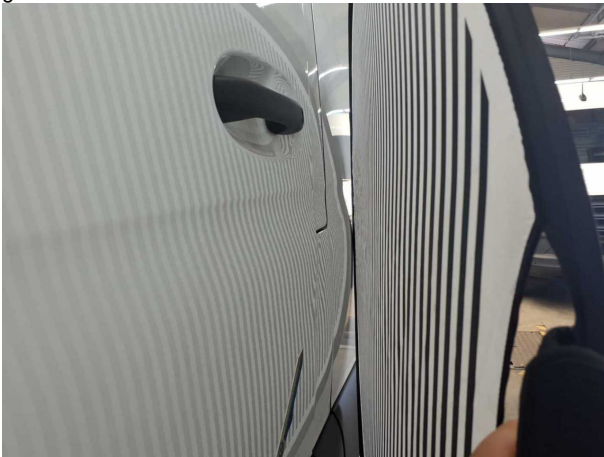
Beschädigung #2: Tür vorn links: Tür - verformt - Smart Repair
