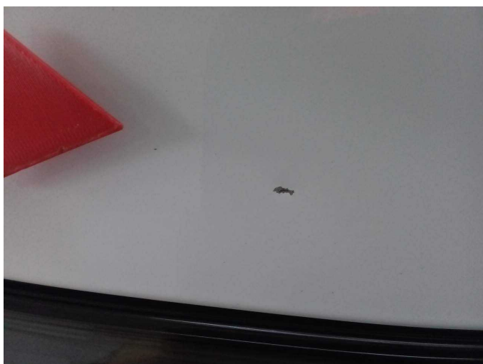
Damage 12: Bonnet: Bonnet - Dent / paintcoat damage - Repair and paint
