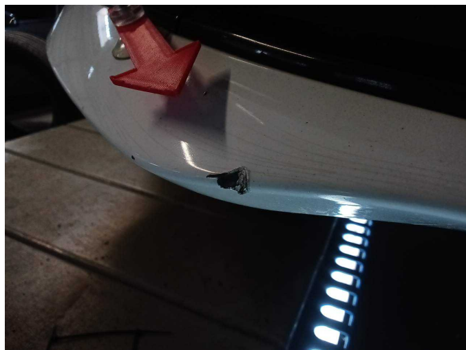
Damage 11: Front bumper: Spoiler - Scratched - Repair and paint
