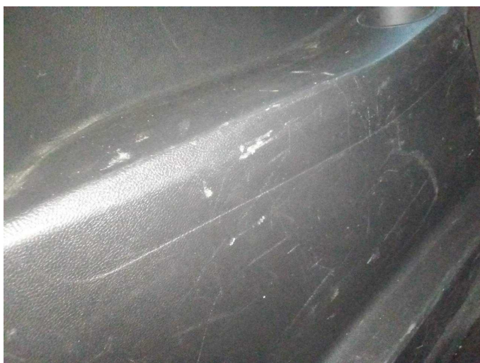
Damage 9: Trim / covers: Boot lining - Scratched - Loss in value
