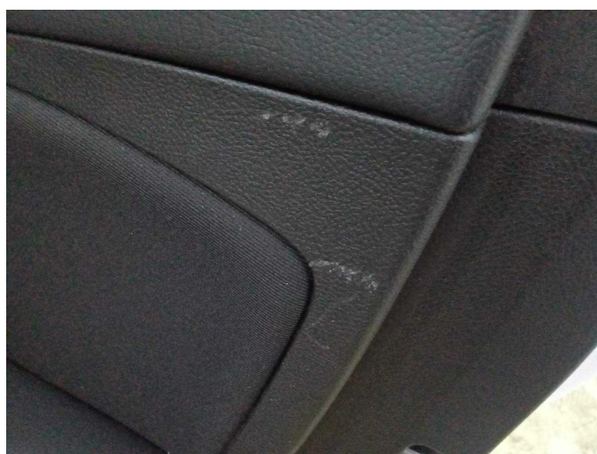
Damage 4: Trim / covers: Door trim - rear right side - Scratched - Smart repair
