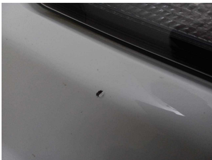
Damage 8: Front bumper: Front bumper - Stone chips - Smart repair
