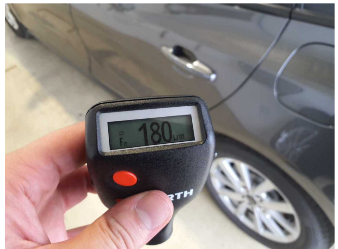
Repainting 3: Door - rear left side
