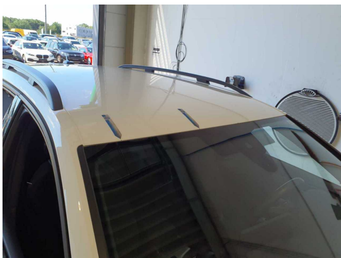
Damage 3: Roof: Roof (Dachkante) - Corrosion - Paint
