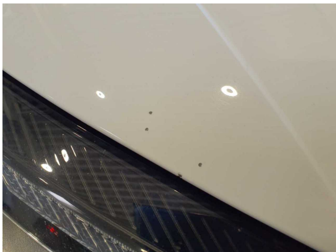
Damage 2: Bonnet: Bonnet - Corrosion - Paint
