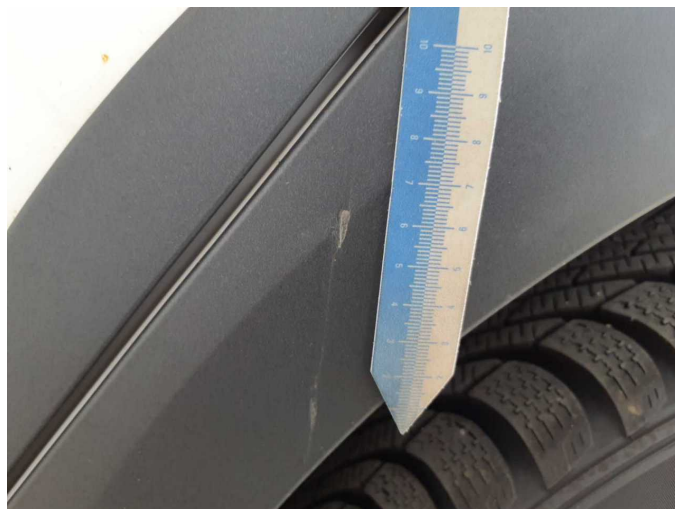
Damage 1: Side panel - rear left side: Wheel well extension - Scratch(es) - Replace
