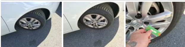
Tyre FR, Out of tolerance, Replace
