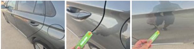
Door FL, Scratch(es), Repair and paint (complete)
