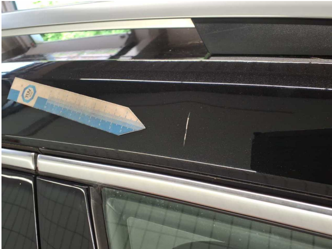
Damage 9: Roof: Roof (+ Dachholm re.) - Dent / paintcoat damage - Repair and paint
