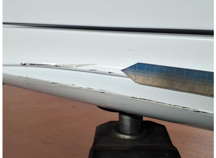
Damage 5: Sill - right side: Trim - Scratched - Paint
