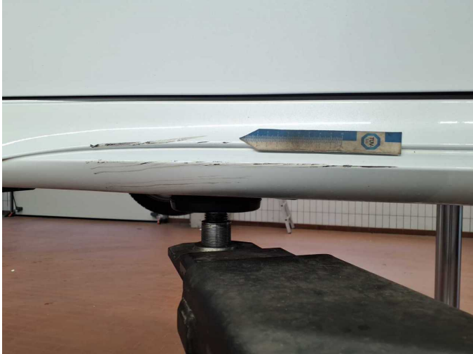
Damage 5: Sill - right side: Trim - Scratched - Paint
