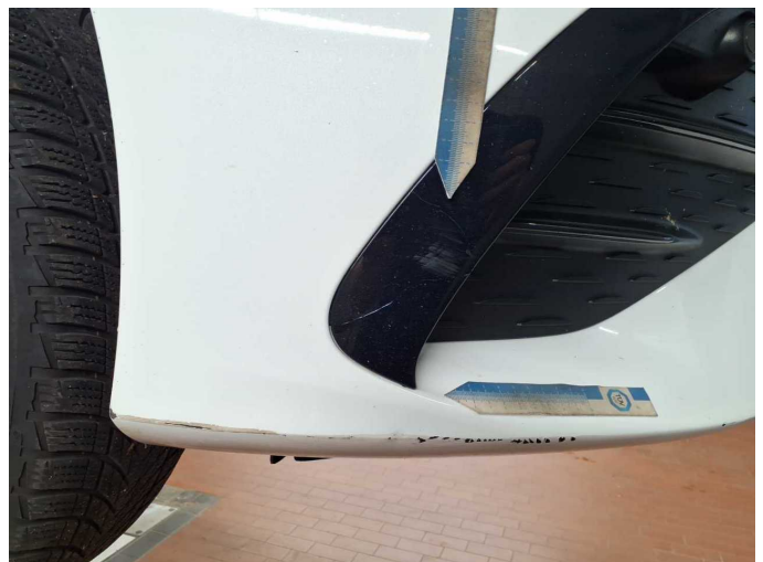
Damage 6: Front bumper: Front bumper (+ Blende rechts gebrochen erneuern) - Scratched - Repair and paint
