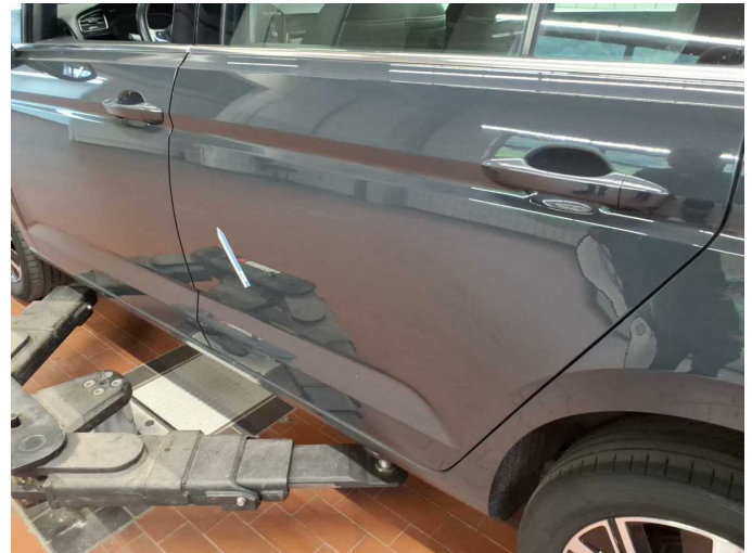
Damage 5: Door - rear left side: Door - Dent / paintcoat damage - Repair and paint
