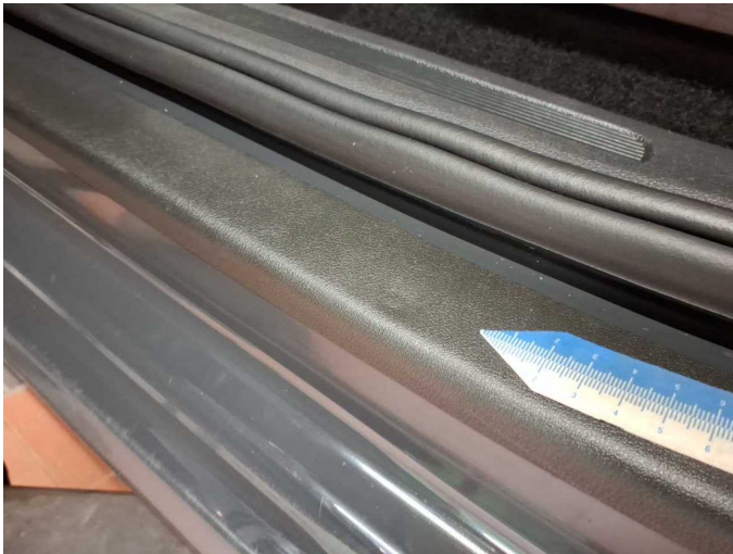
Damage 4: Side panel - rear left side: Sill (Folie überklebt dellen/ Lackschaden) - Dent / paintcoat damage - Repair and paint
