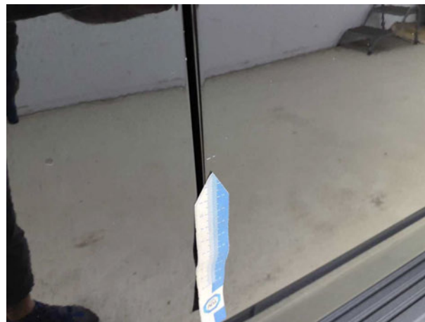
Beschädigung #1: Tür hinten links: Tür - Kratzer - Smart Repair
