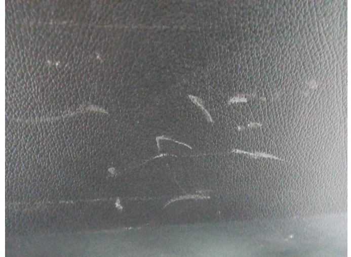
Damage 6: Trim / covers: Boot lid - interior trim - Scratch(es) - Smart repair
