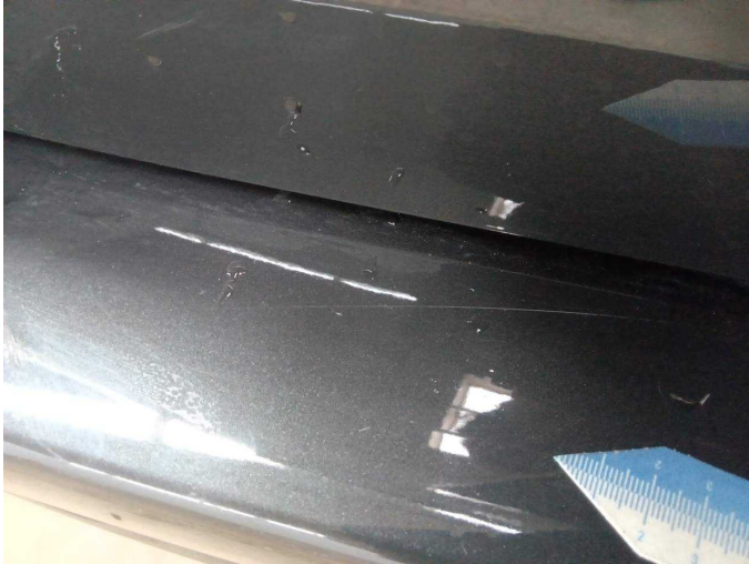
Damage 10: Rear bumper: Rear bumper - Scratch(es) - Paint
