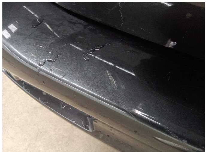
Damage 10: Rear bumper: Rear bumper - Scratch(es) - Paint
