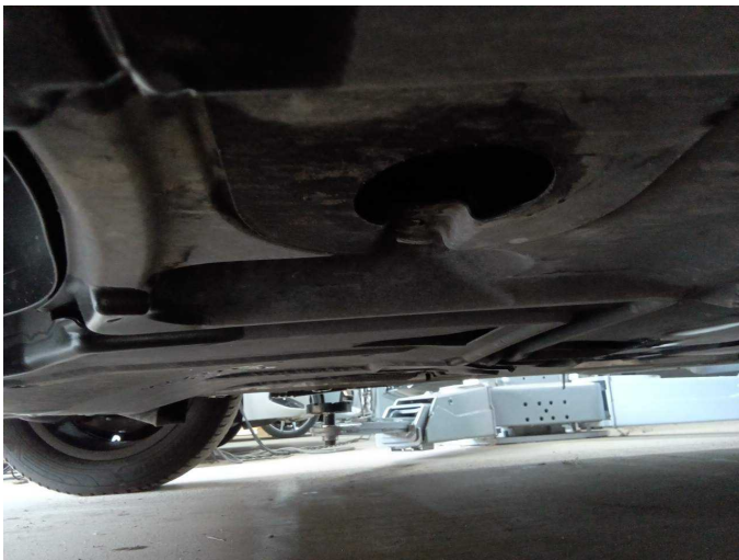
Damage 2: Sill - left side: Jacking point - front - Damaged - Replace
