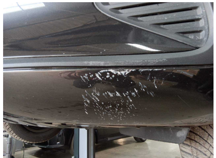
Damage 12: Front bumper: Front bumper - Scratch(es) - Paint
