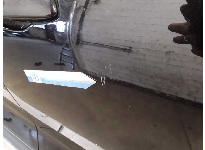
Damage 4: Door - front right side: Door - Scratch(es) - Smart repair
