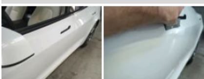
Outer sill L, Dent(s) and scratch(es), Repair and paint (complete)
