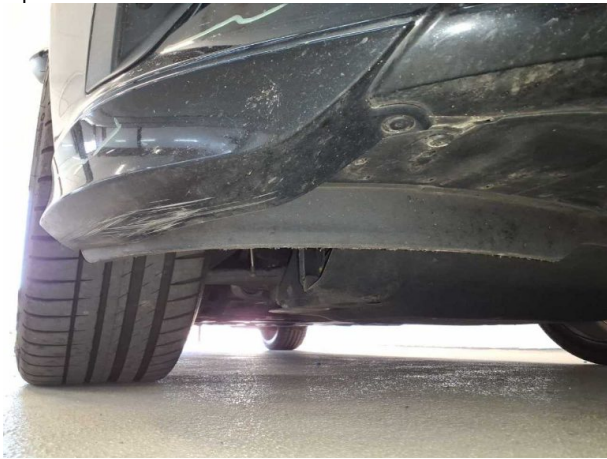
Damage #10: Front bumper: Front bumper - Scratched - Smart repair
