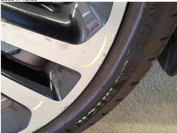
Damage #9: Wheel / tyres: Alloy rim - rear right side - Scratched - Loss in value
