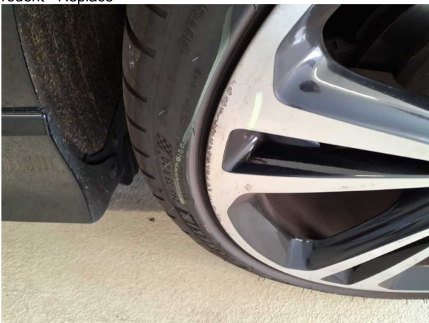
Damage #6: Wheel / tyres: Alloy rim - rear left side - Scratched - Loss in value
