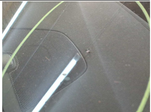
Damage #12: Vehicle glazing: Windscreen - Stone chips - Replace
