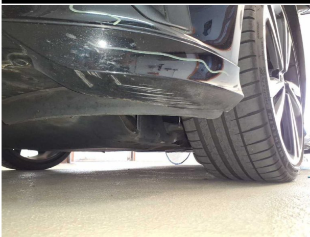
Damage #10: Front bumper: Front bumper - Scratched - Smart repair
