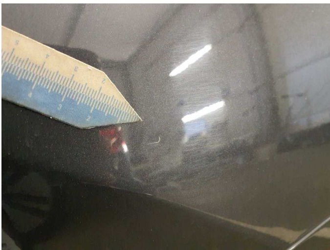
Wear and tear 1: Side panel - rear left side: Side panel - dent(s) - Smart repair
