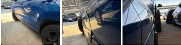
Door FL, Dent(s) and scratch(es), Repair and paint (complete)
