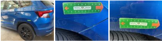
Door RL, Dent(s), Repair and paint (complete)
