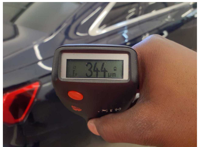
Repainting 1: Side panel - rear right side
