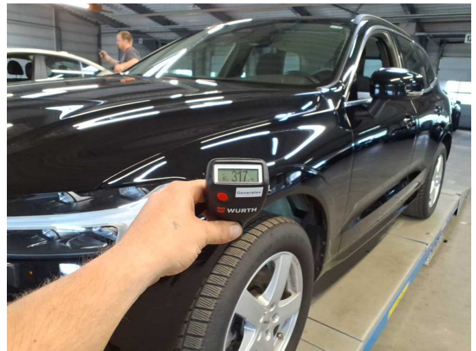
Repainting 1: Mudguard - left side
