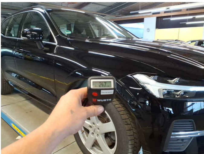
Repainting 2: Mudguard - right side
