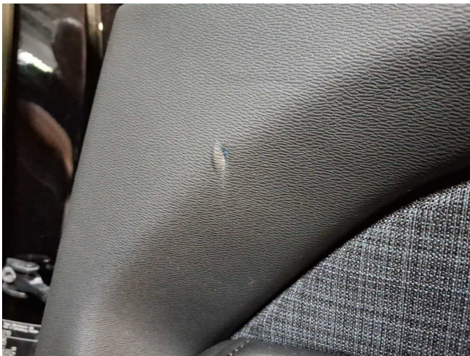
Damage 2: Trim / covers: Door trim - rear right side - Broken / torn - Replace
