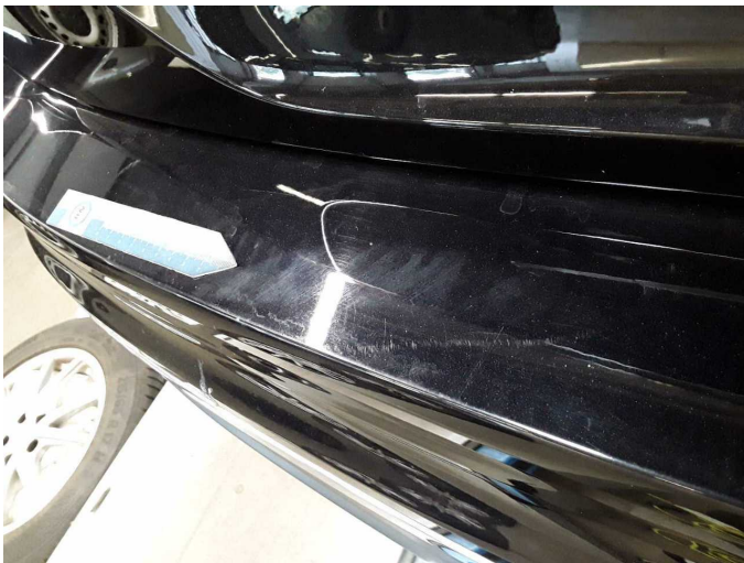
Damage 5: Rear bumper: Rear bumper - Scratch(es) - Paint
