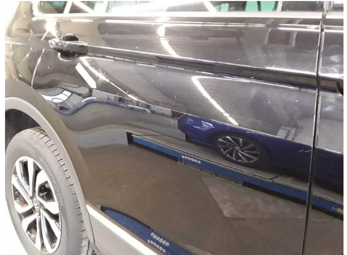
Damage 7: Door - rear right side: Door - Dent / paintcoat damage - Repair and paint
