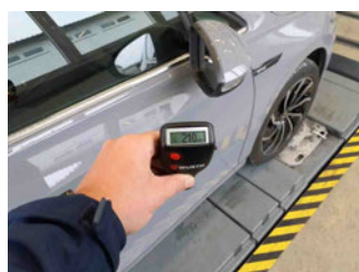
Paint thickness Door FR
