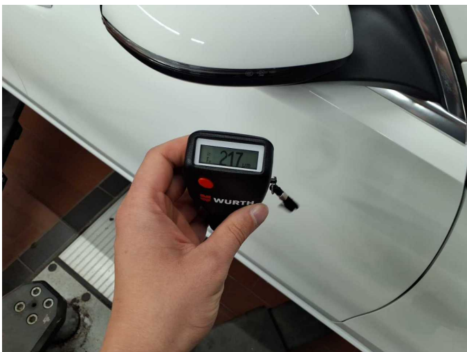
Repainting 2: Door - front right side
