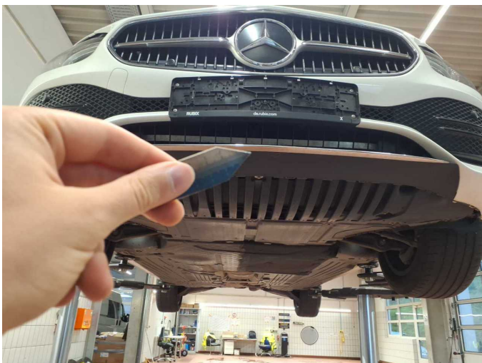
Damage 5: Front bumper: Spoiler (+ Chromleiste) - Scratched - Replace
