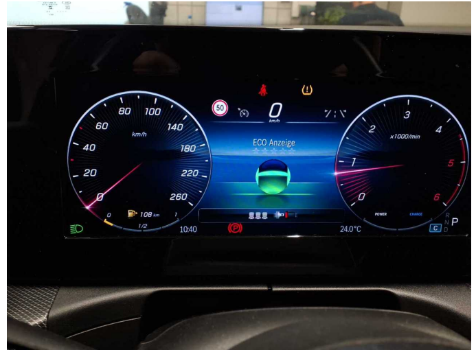
Damage 1: Instrument panel: Indicator light (Reifendruckkontrollsystem) - Electrical fault - Perform diagnosis
