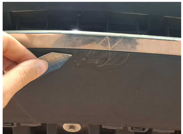
Damage 5: Front bumper: Spoiler (+ Chromleiste) - Scratched - Replace
