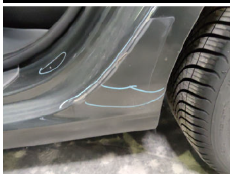
Kotflügel / Hinten Links / Delle
