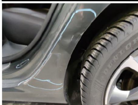
Kotflügel / Hinten Links / Delle
