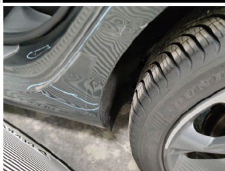
Kotflügel / Hinten Links / Delle
