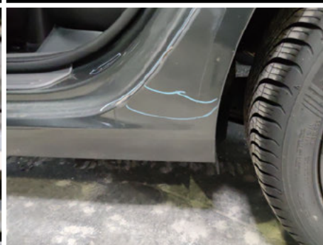
Kotflügel / Hinten Links / Delle
