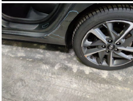
Kotflügel / Hinten Links / Delle
