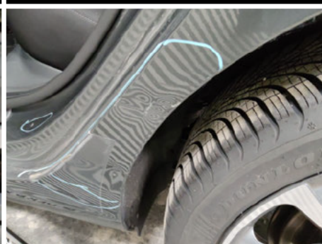
Kotflügel / Hinten Links / Delle
