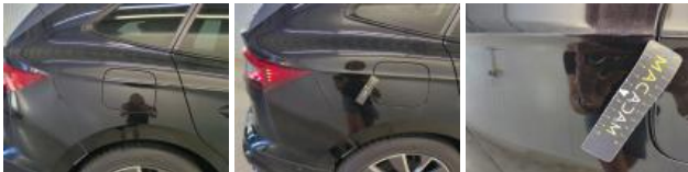
Door RR, Dent(s), Repair and paint (complete)
