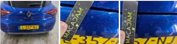
Tailgate / Boot, Scratch(es), Repair and paint (complete)
