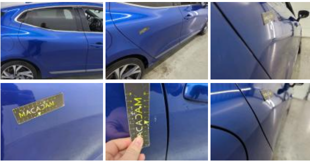
Roof pillar R, Scratch(es), Repair and paint (complete)
