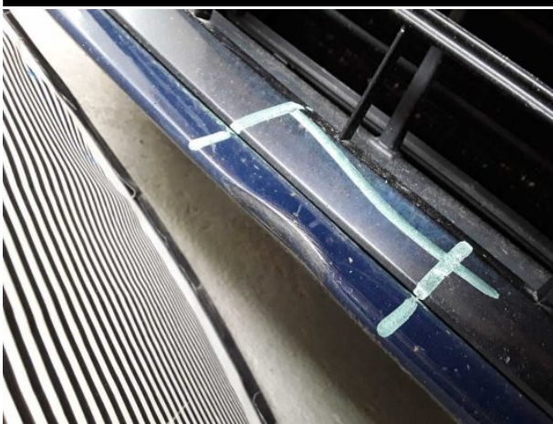
Damage #7: Front bumper: Front bumper - Deformed - Replace
