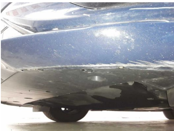
Damage #7: Front bumper: Front bumper - Deformed - Replace
