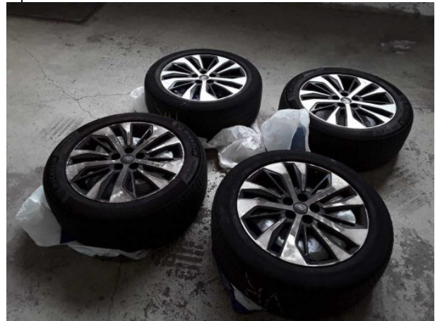
Damage #4: 2nd wheel set: Tyres - complete set - Worn - Replace
