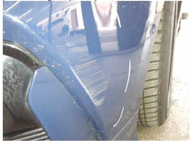
Damage #7: Front bumper: Front bumper - Deformed - Replace
