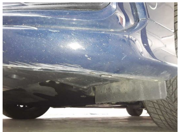
Damage #7: Front bumper: Front bumper - Deformed - Replace
