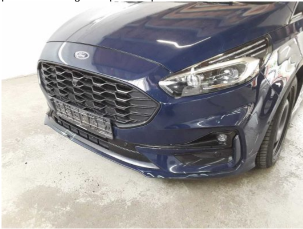
Damage #7: Front bumper: Front bumper - Deformed - Replace
