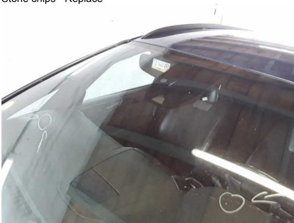
Damage #8: Vehicle glazing: Windscreen, heated (Rissbildung) - Stone chips - Replace
