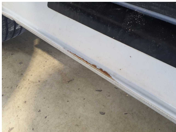
Damage 7: Sill - left side: Sill - Corrosion - Repair and paint
