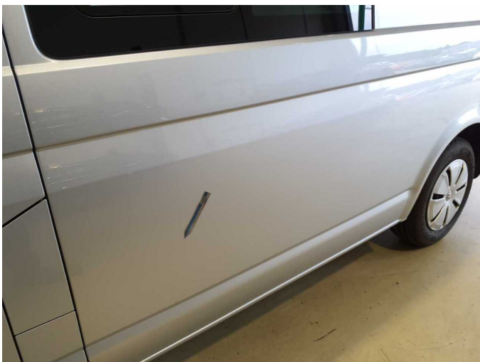
Damage 13: Side panel - rear left side: Side panel (Einschlüsse) - Unprofessionally repaired - Repair and paint
