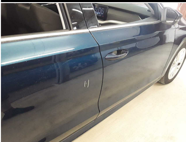
Damage #3: Door - front right side: Door - Scratched - Repair and paint
