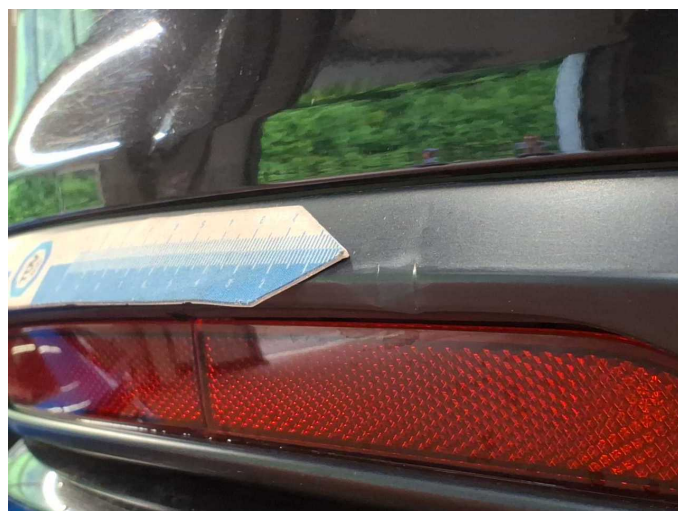
Damage 10: Rear bumper: Spoiler - dent(s) - Replace
