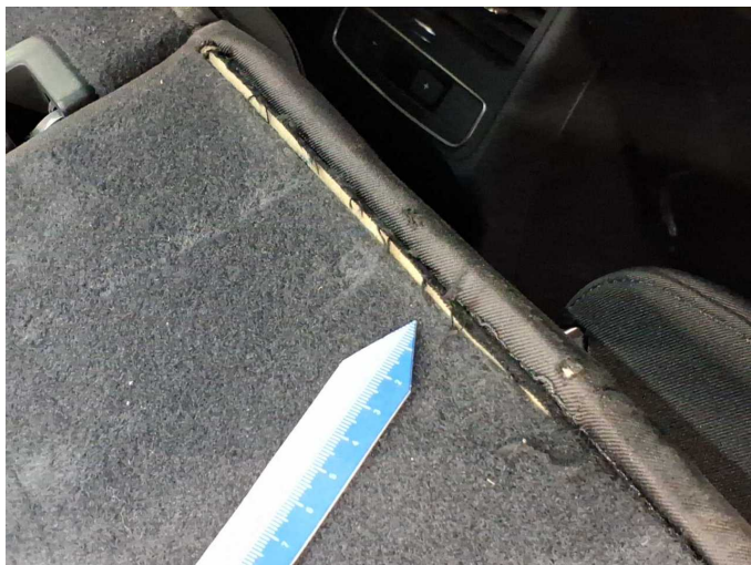
Damage 13: Seat - rear: Backrest cover - Broken / torn - Replace
