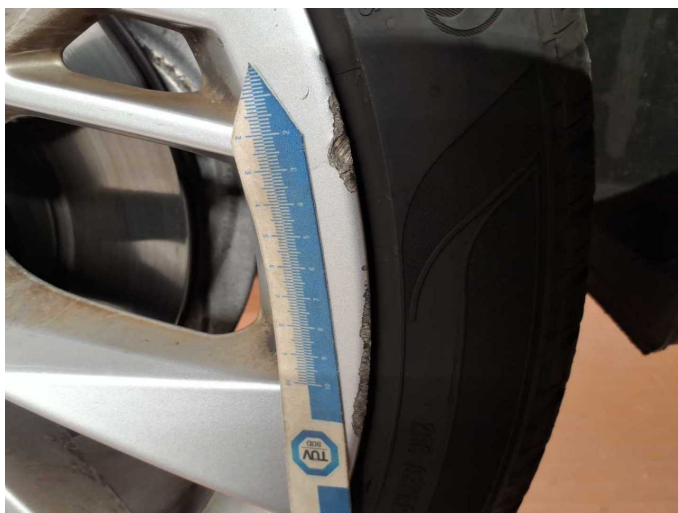
Damage 14: Wheel / tyres: Alloy rim - front right side - Scratched - Replace
