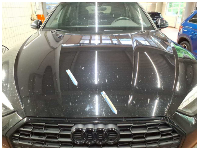
Damage 18: Bonnet: Bonnet - Stone chips - Paint
