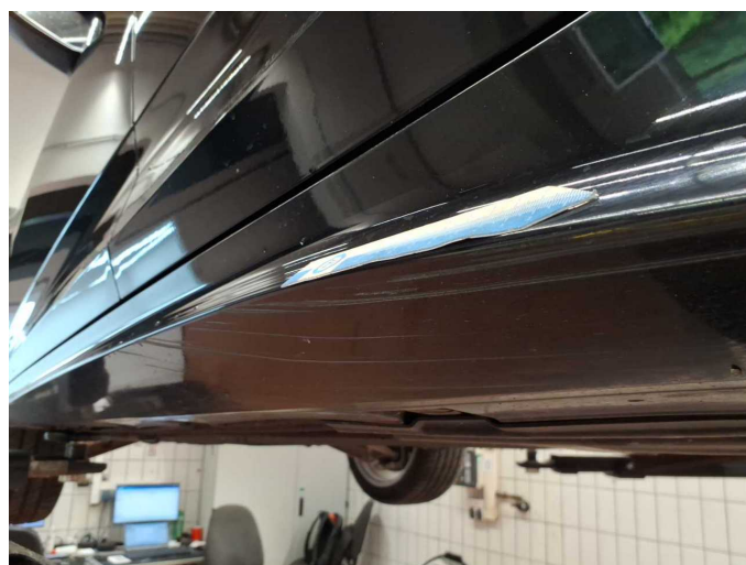
Damage 11: Sill - left side: Trim - Scratched - Paint
