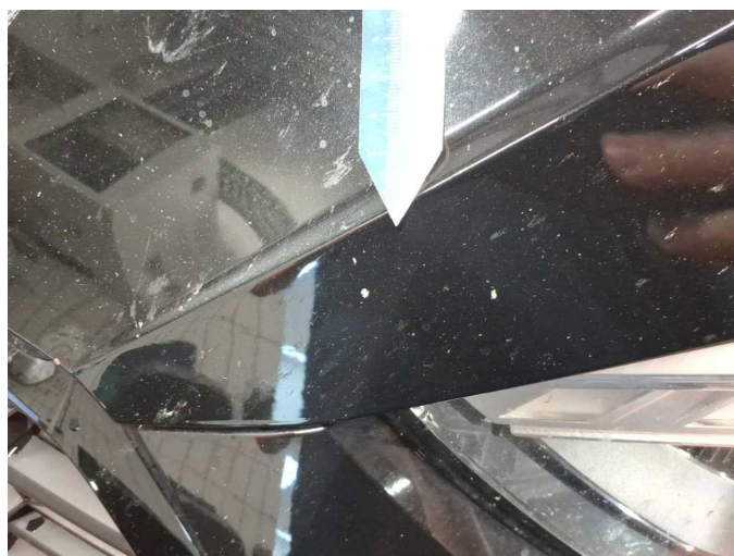
Damage 18: Bonnet: Bonnet - Stone chips - Paint
