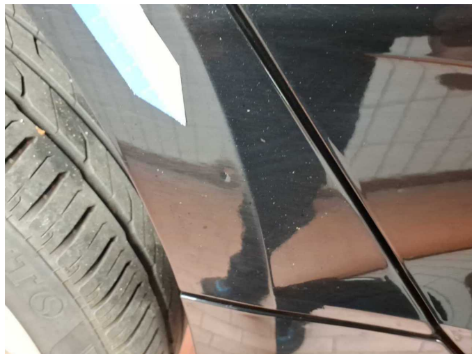
Damage 15: Side panel - rear right side: Side panel - Dent / paintcoat damage - Repair and paint
