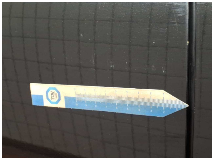
Damage 17: Door - rear right side: Door - Scratch(es) - Paint
