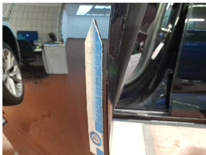
Damage 7: Door - front left side: Door edge - Scratch(es) - Smart repair
