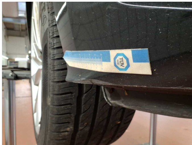
Damage 19: Front bumper: Front bumper - Scratched - Paint
