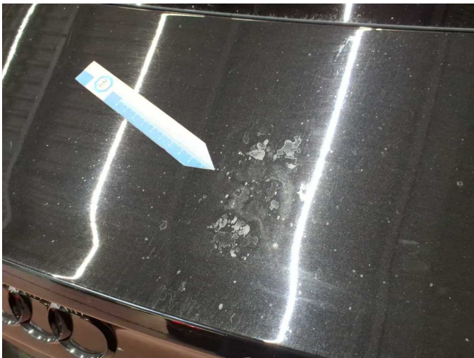
Damage 4: Boot lid / rear door: Boot lid - Soiled - Conditioning
